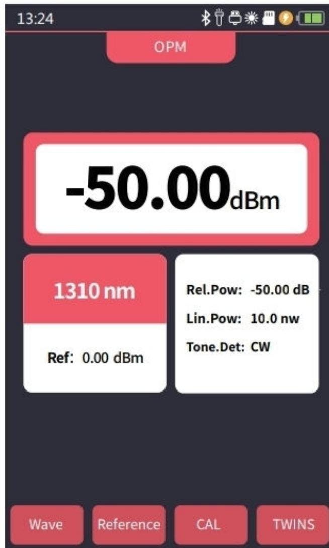
The function is used to test the power of optical signal and insertion loss of various devices and photoelectric components. It can identify and measure the frequency of 270/330/1000/2000Hz optical signal.
