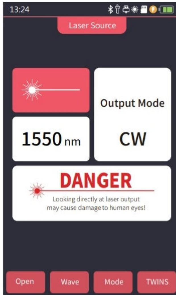
The wavelength of stabilized laser source is the same as OTDR wavelength. It is used to measure the parameters of telecommunication, CATV, LAN cable, insertion loss, isolation loss and echo loss of optical passive devices, and wavelength responsiveness of detectors.
